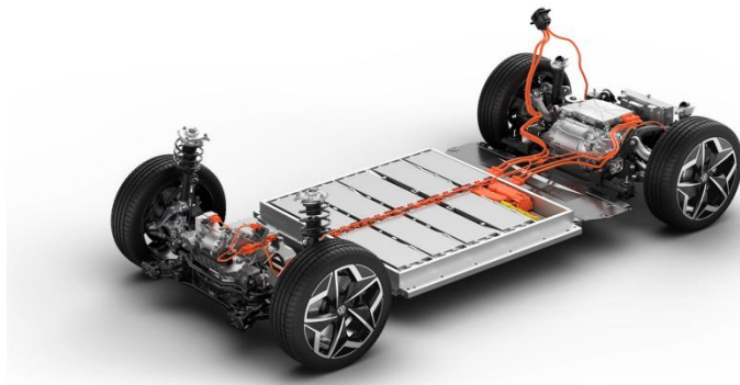
Figure 8: Location of the battery in the EV
