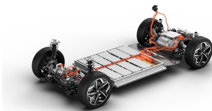
Figure 9 Location of the battery in the EV
