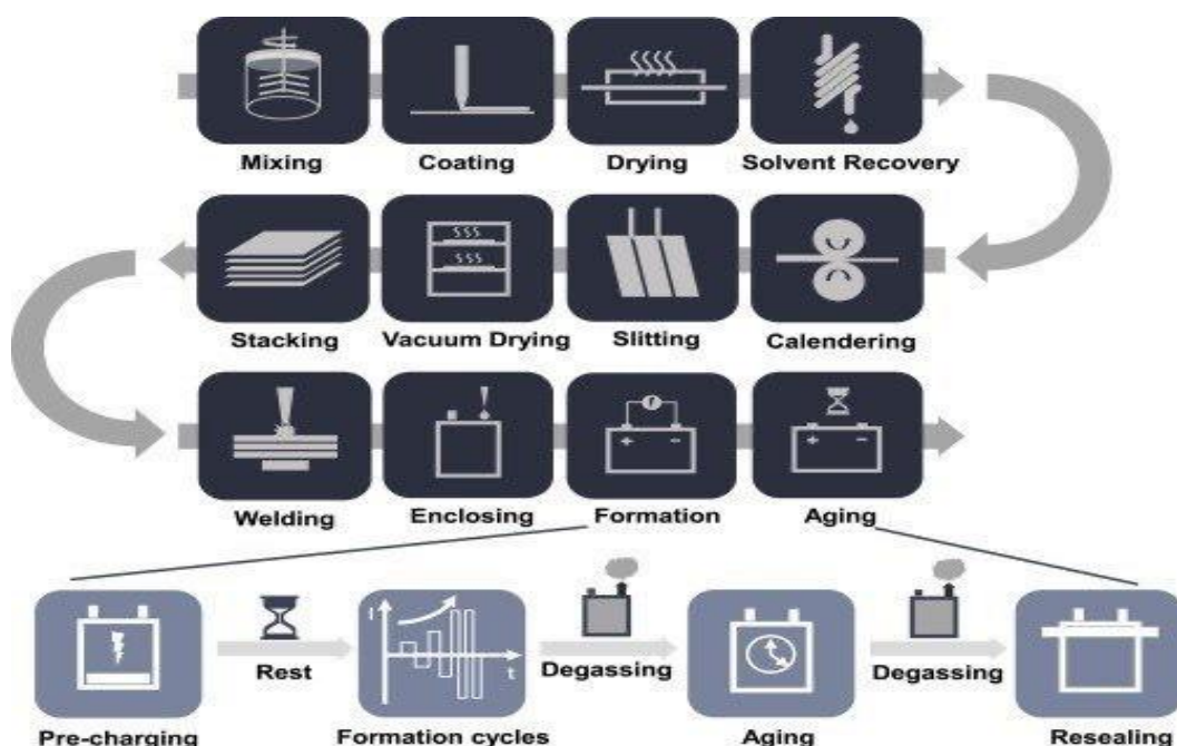
2. Battery manufacturing flow chart
